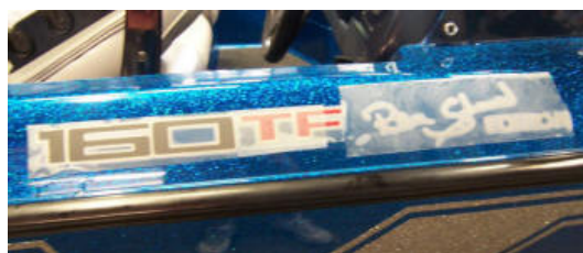
New Model Designator Decal (transfer tape still on - drying stage)
